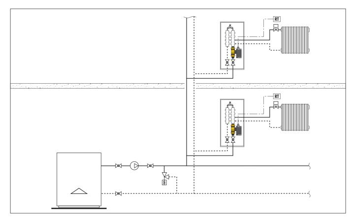
System with 2-way zone valves, variable speed pump and Autoflow
