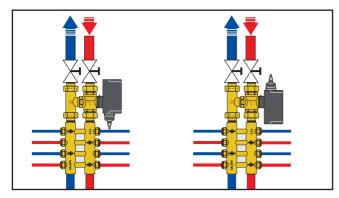
The actuator can be mounted on the valve body in the two positions indicated, vertical or horizontal. Fixing is via a stainless steel clamp ring.
