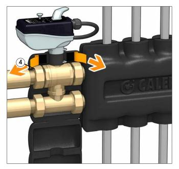
The 6459 series insulation (flow / return) must be used with the 6453 series valve when coupled to the 6459 series by-pass tee to be all together connected to the the 356 ... IS series cast monoblock dual distribution manifold. This assembly requires to eliminate the insulation supplied with the valves. The self-sticking labels (4) enable a quick fitting of the insulation without using fixing glues.
