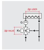
In a mixing circuit, the portion upstream from the three-way valve is usually a zone with negligible  $\Delta \rho$  (and there is normally a hydraulic separator). Therefore the main pressure drop is due to the three-way valve, giving it regulating authority. For this reason, the three-way valve can be dimensioned by considering an acceptable pressure drop for the user circuit pump, which indicatively may be from 5 % to 15 % of the pressure drop in the user circuit:
