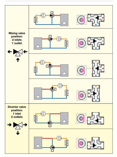
**DIVERTING CIRCUIT (flow rate control)**
