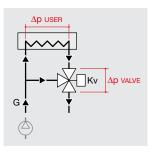
In these two types of circuit, the two- or three-way diverter valve regulates the flow rate passing through the user circuit. In such cases, it is important to have good authority by dimensioning the regulating valve to ensure that the pressure drop is not too low compared to that of the user circuit. Recommended values for rapid sizing can be chosen considering:
