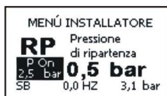
Figure 14: Setting the restart pressure
