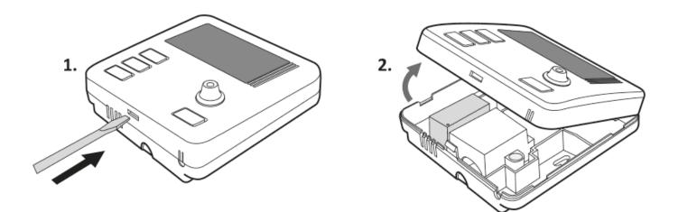
The terminals are located on the back of AURATON Libra DS, under the plastic casing.
