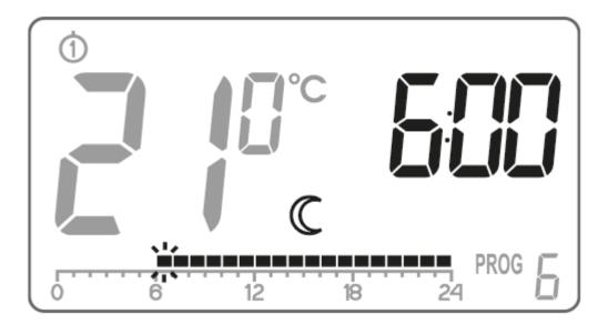
By pressing the  $\textcircled{\sc c}$  key and selecting time interval the entire program is modified.
