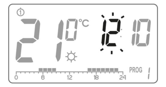
Turn the knob to the left or right to set the required hour and confirm with using the  $\Box$  button.
