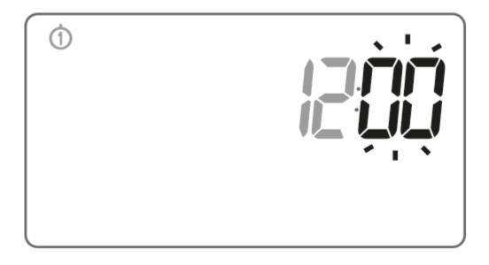
A flashing symbol of the day of the week appears in the upper left corner. Turn the knob to the left or right to set the day and confirm the selection using the  $\Box$  button.
