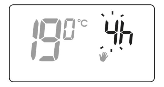
3. The temperature field starts flashing. It can be set with the bc buttons. Confirm the selection with the i button.
