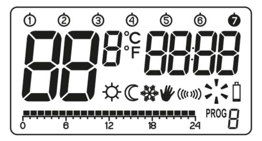
After a while, AURATON Tucana will automatically go to the hour setting. An item flashing on the screen indicates that it is currently in editing mode. Use the bc buttons to set the desired hour and confirm the setting with the i button.
