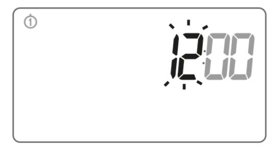
AURATON Tucana will go to the minute setting. Use the bc buttons again to set the desired minute value and confirm the setting by pressing the i button.
