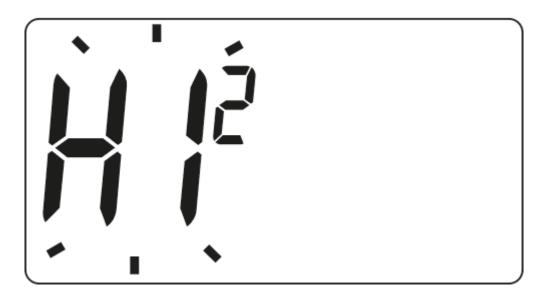
The hysteresis change mode is signaled by a flashing  $\mathbf{HI}$ . Use the **bC** buttons to set the desired hysteresis.
