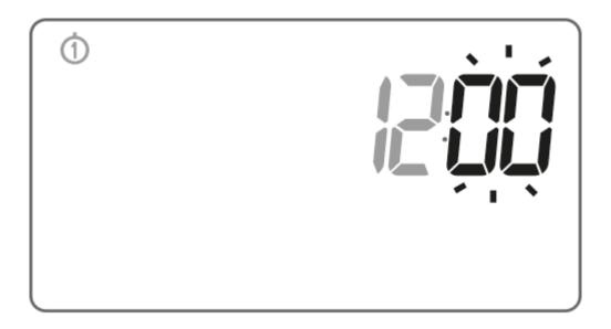
A flashing day of the week symbol appears in the upper left corner. Use the bc buttons to set the desired day and confirm the selection with the i button. AURATON Tucana will enter its normal operating mode.
