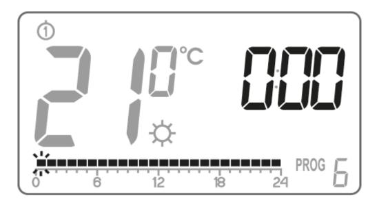
Press the ; or : button to select the day temperature (a lit rectangle) or the night temperature (no rectangle) on the timeline.
