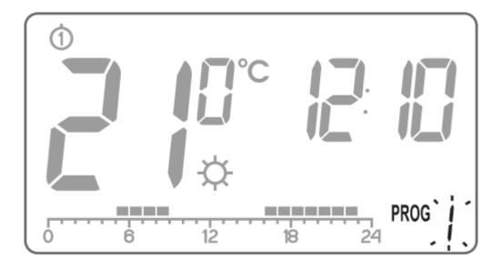
Press the I button. Using the bc buttons or the I button set the day of the week when the program should be executed.
