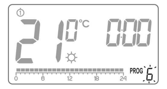
All (24) black rectangles will be lit on the timeline, each symbolising 1 hour. A visible rectangle means that the day temperature is to be achieved during a given hour. No rectangle above the timeline is tantamount to planning the night temperature.
