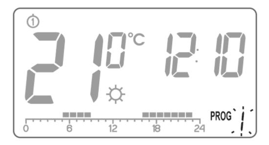
Press the I button. Using the bc buttons or the I button, set the day of the week when the program should be executed.
