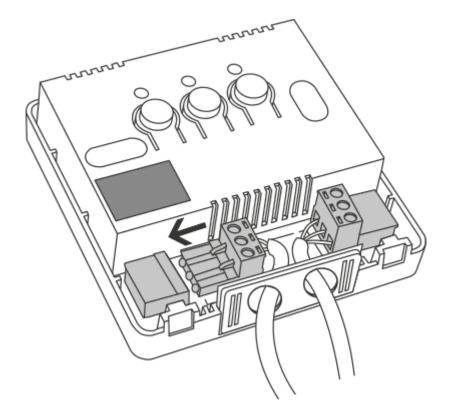
Connect the heating device to the clips of the AURATON Fornax control connector. Follow the service manual of the heating device. COM (common) and NO (normally open circuit) clips are most commonly used.
