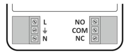
Connect the power supply wires to the clips of the power supply connector of the AURATON Fornax receiver, observing safety rules.
