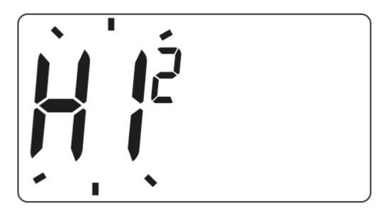
The hysteresis change mode is signaled by a flashing **HI**. Use the **bC** buttons to set the desired hysteresis.
