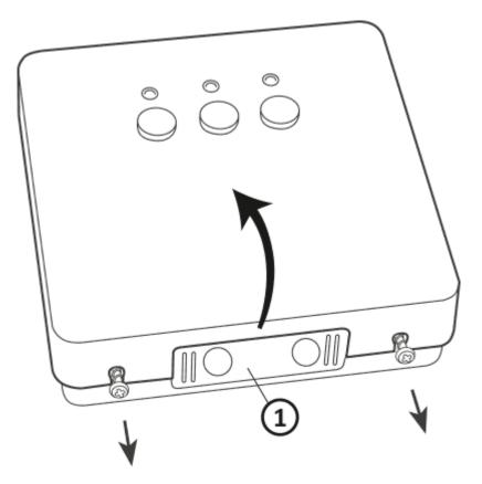
Remove the cover of the front part of Auraton Fornax by unscrewing the screws halfway.
