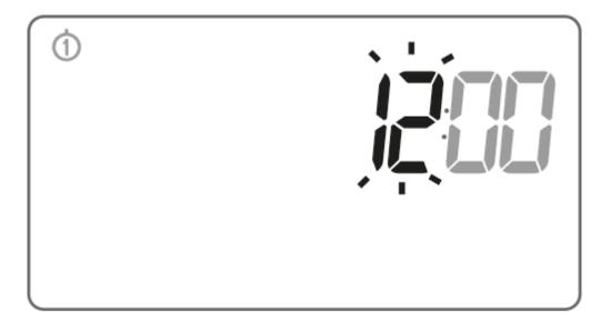
Tucana AURATON will go to the minute setting. Use the bc buttons again to set the desired minute value and confirm the setting by pressing the i button.
