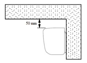
The width of the curtain should be greater or equal to the width of the door frame. When the entrance is wider than the unit, it is recommended to install two or more units in parallel. In this case, provide 10-40 mm gaps between the units.
